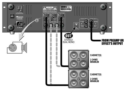
Set the Stereo/Dual Mono / Mono Bridge switch to the Stereo/Dual Mono position (switch out).
